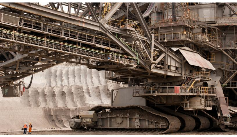
The largest excavators in the world are used in open-cast mining. Because they weigh over 10,000 tonnes, they run on tracks/caterpillars. (© corlaffra / Shutterstock.com).
