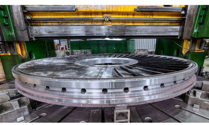
The components of a turbine are large, round, and heavy and must be precisely manufactured. This is best done on a vertical turret lathe. (© Nordroden / Shutterstock.com).
