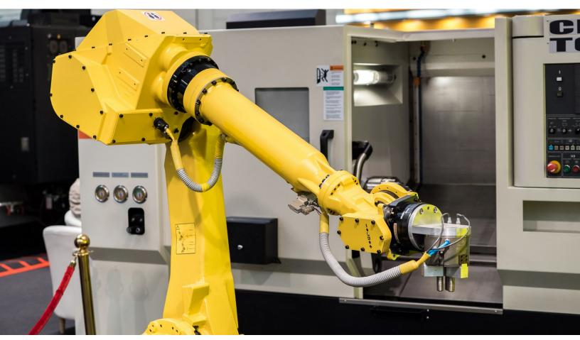
Industrial robots can also be retrofitted in current machinery. A robot can take charge of placement and workpiece handling for automated production with CNC machines. (© Alexander Tolstykh / Shutterstock.com).
