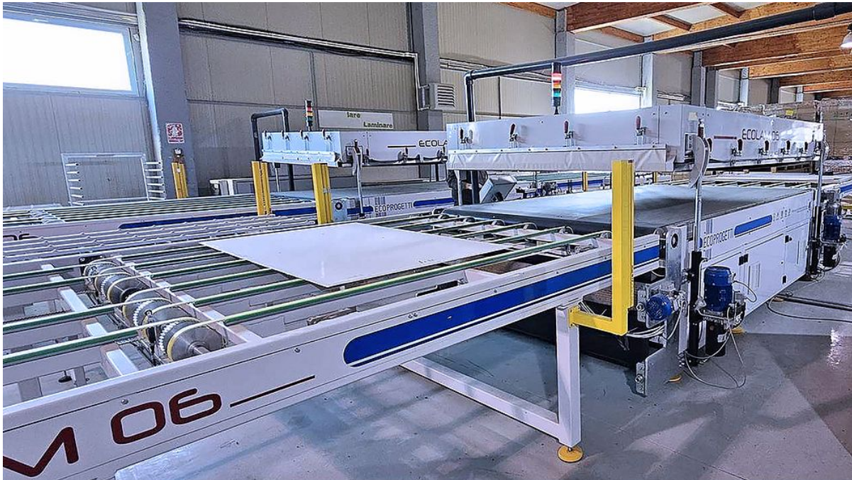
During lamination, the individual layers of the module—glass, EVA, strings, and encapsulation materials—are fused into a single unit. (© Surplex).
