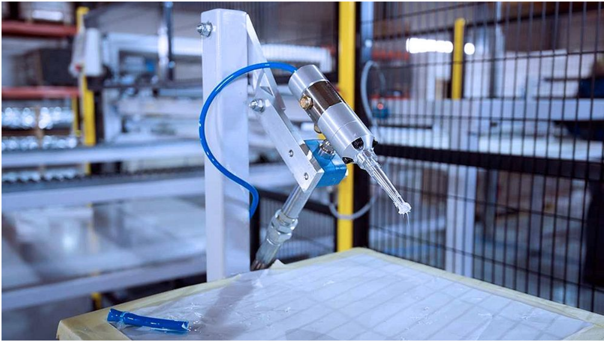
Precision silicone application ensures a secure aluminium frame attachment to the solar module. (© Surplex).
