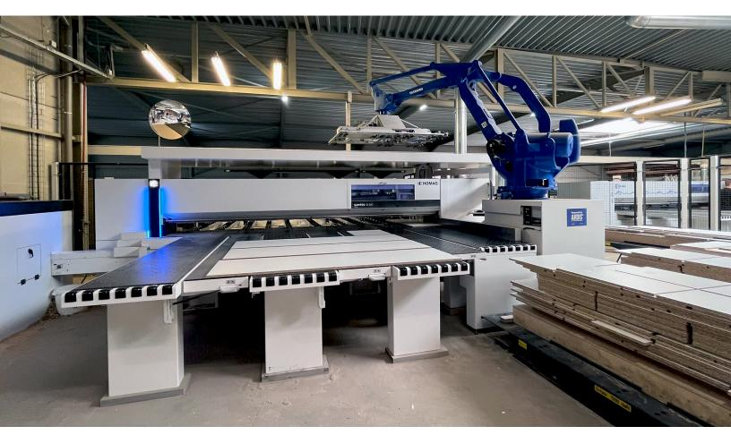
Robots take on tasks such as loading the saw, turning and positioning the boards, and stacking the finished cuts. (© Surplex).
