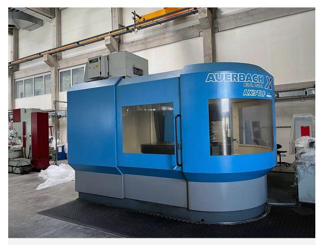
Plastics manufacturers rely on precise metal processing machines for mould making—which is why this auction also includes high-quality CNC milling and drilling machines. Pictured: AUERBACH AX3 TLF CNC deep hole drilling machine. (© Surplex).
