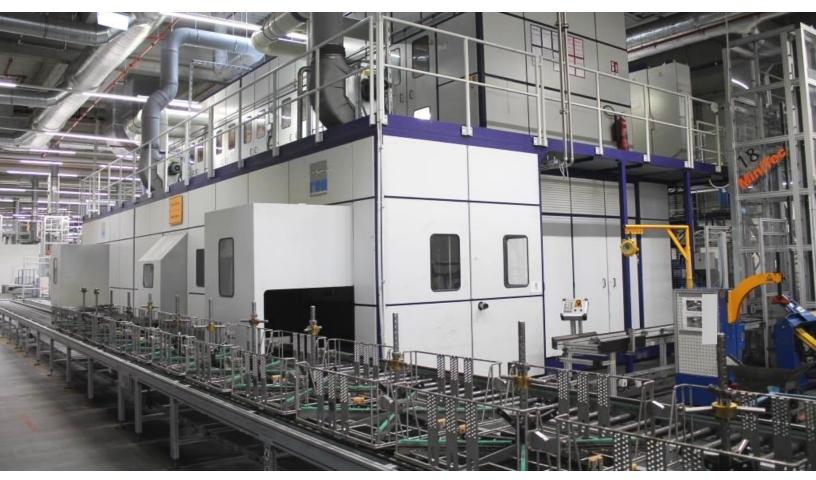
An automatic cleaning system enables aircraft rims to be easily and quickly made ready for use. (© HT).
